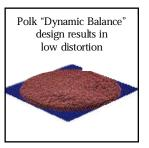
Laser Interferometry tests produced holographic "photos" of drivers in motion. The "bad" drivers are experiencing modal breakup that results in performance-robbing resonances. A "perfect" driver would look like a cake (flat on top), more, like the photo on the right.
